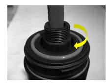
7. Install the Strain Relief (push on) over the cable and tighten the Clamp Screw. Cut and remove the outer jacket and braid to the top of the strain relief. **Do not cut through to inner jacket.**
