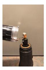
11. Turn the Cap Light Assembly 2 complete turns counterclockwise and thread the Cap Assembly (clockwise) onto the Stanchion. Secure the completed assembly with the supplied Tie Wrap.
