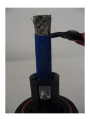
**11.** Slide the Silicon Boot over the end of the cable. Ensure the lower O-ring is in place.
