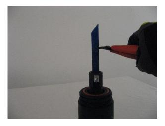
**10.** Trim / remove the outer jacket and ground braid 0.5" (13 mm) from the end of the cable.
