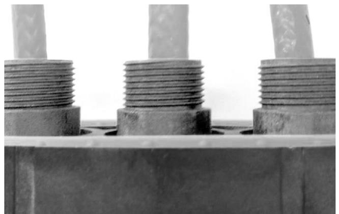
7. Cut outer jacket flush with connector and remove.
